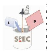
The liquid should be poured into a 20 litre plastic or metal drum. The powder should be added slowly whilst mixing with a spiral paddle attachment on a slow speed electric drill.
